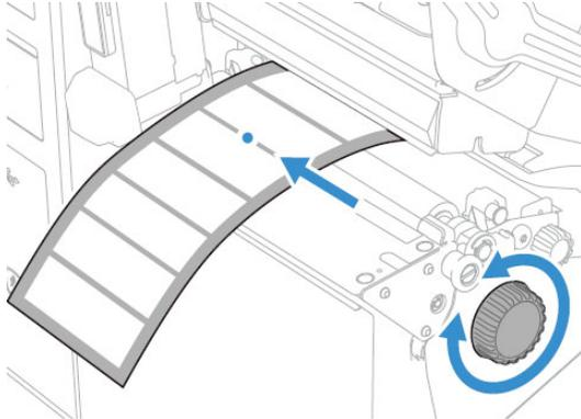
8. Turn the printhead lift lever clockwise to close the printhead and lower the front arm and click into place.
