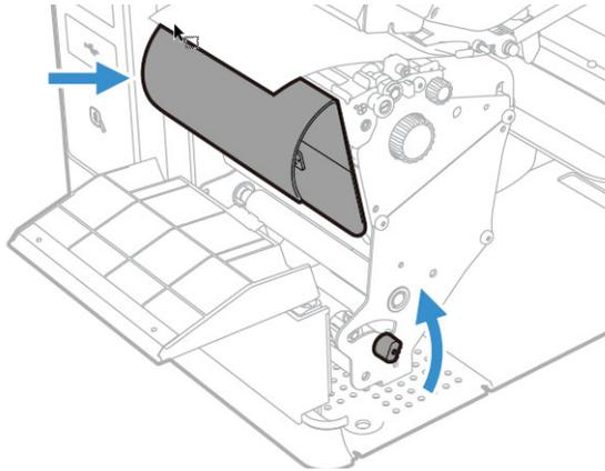
2. Insert an empty media core onto the rewriter take-up hub.
