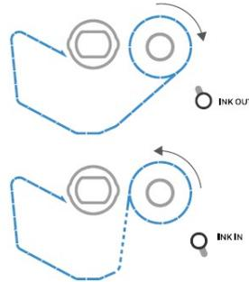
5. Turn the ribbon take-up hub counterclockwise until the ribbon becomes tight and runs wrinkle-free through the print mechanism.
