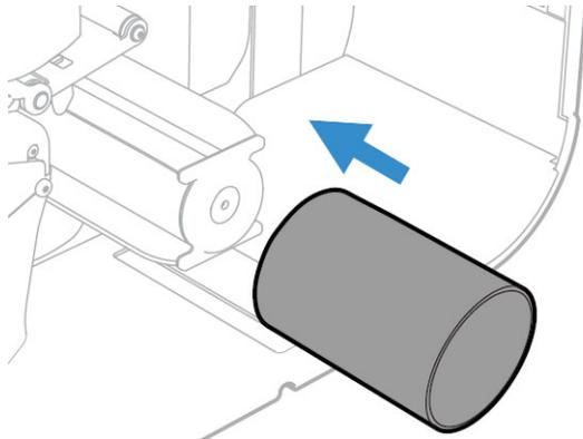
3. Round the liner through the media rewriter and tape leading edge of label to the empty media core to secure position.
