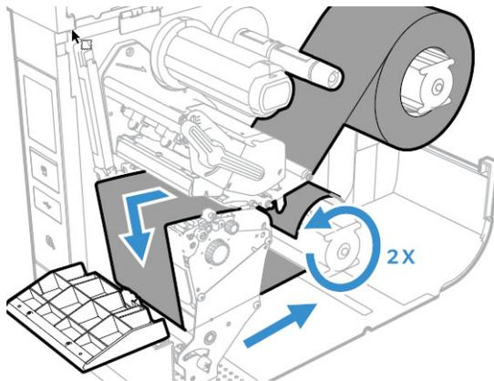
4. Pull the liner tight and lock the Rewind/Liner Take-Up knob into closed position.
