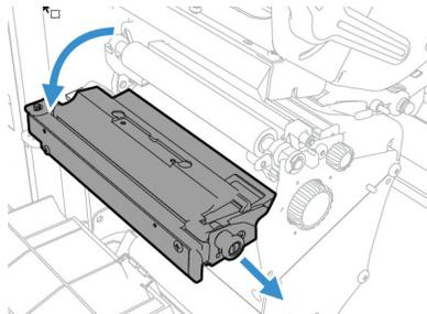
7. Rotate the platen roller latch clockwise to detach it from the printer and pull the platen roller away from the printer.
