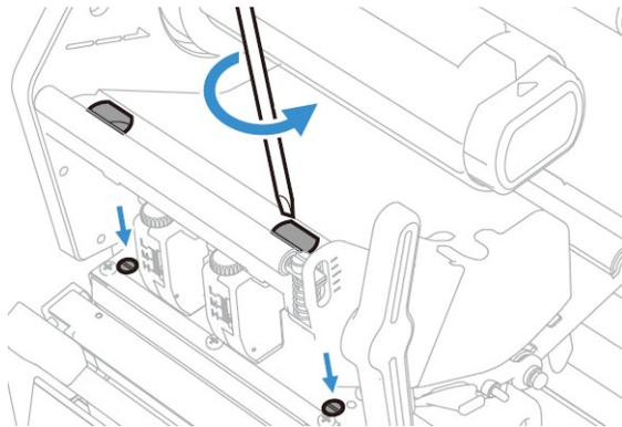
**Note:** Use a long screwdriver and the guiding holes to access the screws.
