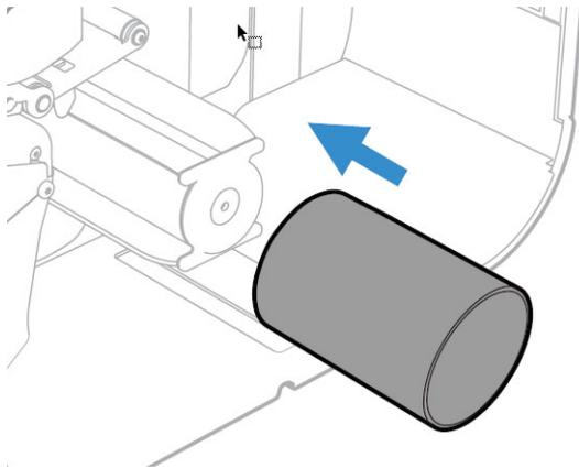
3. Round the media through the rewriter batch plate and tape leading edge of label to the empty media core to secure position.
