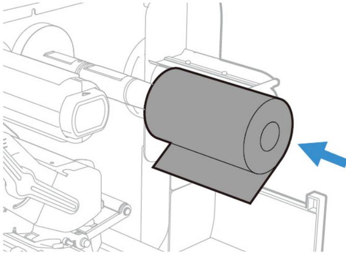
**Note:** For ribbon that has the ink wound out, place the ribbon on the ribbon supply hub with the ribbon wound clockwise. For ribbon that has the ink wound in, place the ribbon on the ribbon supply hub with the ribbon wound counterclockwise.
