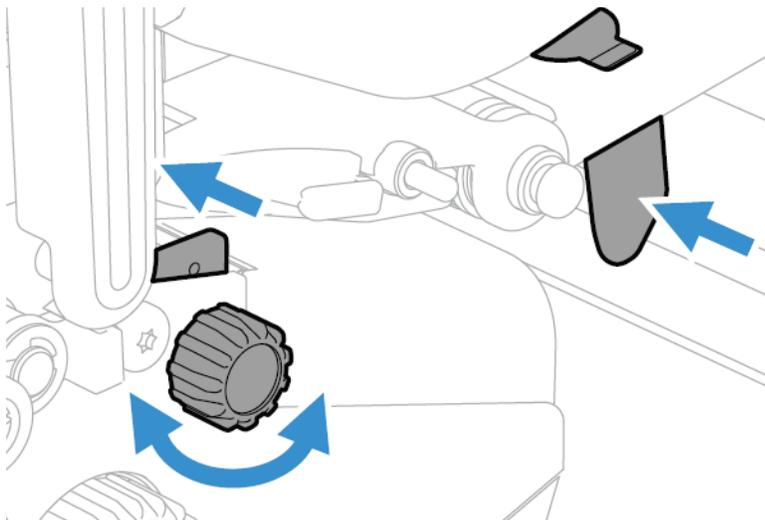
**Note:** There is a media guide that is located near the printhead. It is recommended to adjust the media guide all the way to the right in order to insert the media. If not, it can be difficult to load the media.
