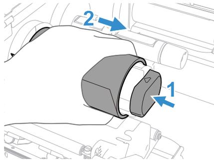
**Note:** Do not push the ribbon release knob in if you do not want to remove the used ribbon as this will cause difficulty to remove ribbon when full.
