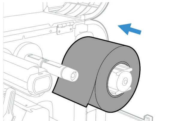
4. Insert the media roll holder and tighten the screw.
