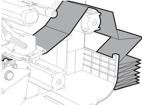
To load Fanfold media from bottom access slot:
